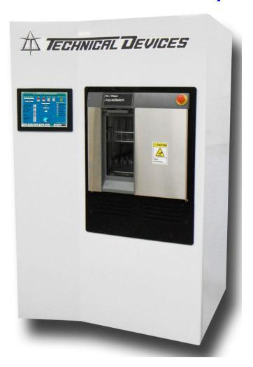
An automatic cleanliness tester is a standard feature that regulates rinsing to a programmable cleanliness level through the use of a built-in DI water resistivity monitor. The cleanliness monitor checks DI rinse resistivity and continues to rinse until desired cleanliness is met.
